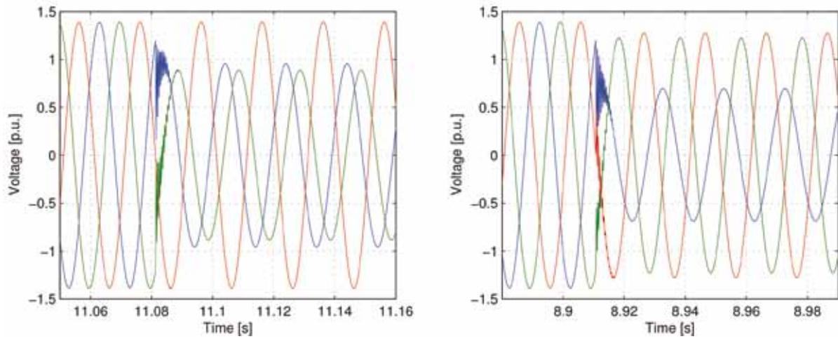
Figure 6. Measured voltages during unbalanced faults. Left: Dd MV/LV transformer. Right: Dy MV/LV transformer.
