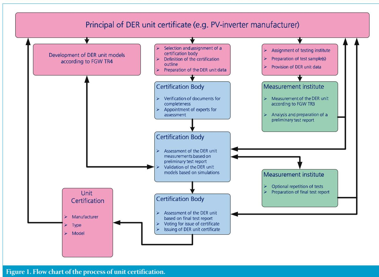
Figure 1. Flow chart of the process of unit certification.
