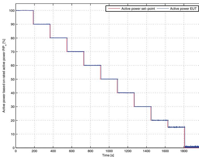
Figure 8. Measurement results for the STP15000TL string inverter with active power reduction by the network operator.
