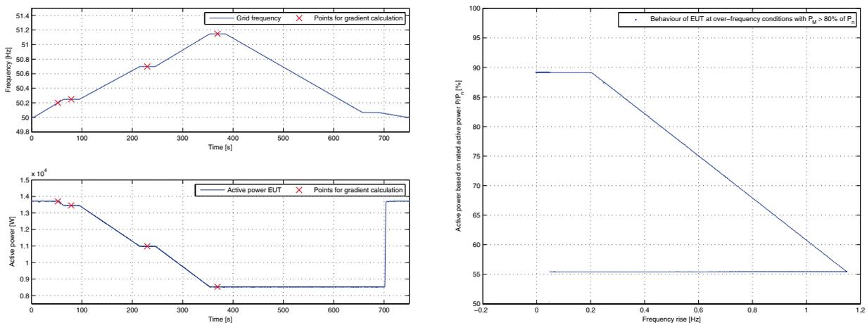
Figure 7. Measurement results for active power reduction corresponding to the over-frequency behaviour of the STP15000TL string inverter.
