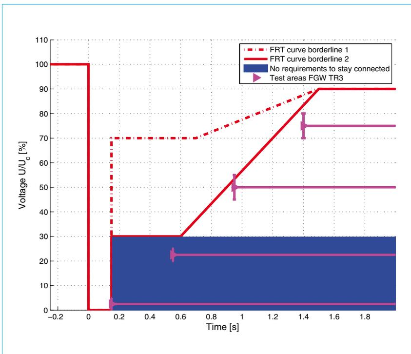
Figure 10. German LVRT curve for type 2 generators, according to [3] and FGW TR3 test areas.
