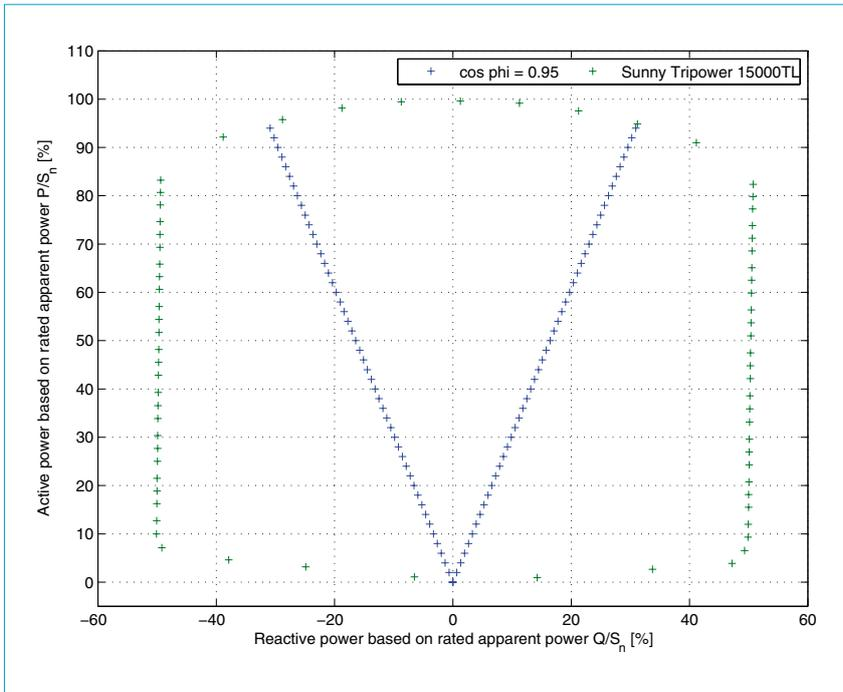
Figure 9. Measured reactive power capability of the STP15000TL string inverter.
