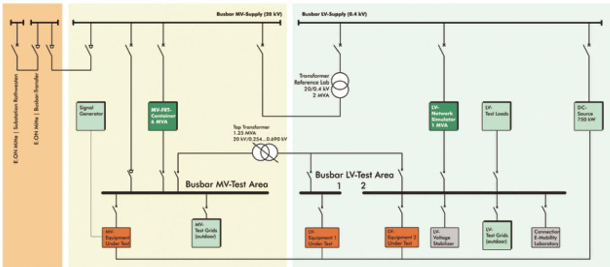
Figure 3. Schematic of the new reference laboratory of Fraunhofer IWES at IWES-SysTec for testing DER units in the higher power range.
