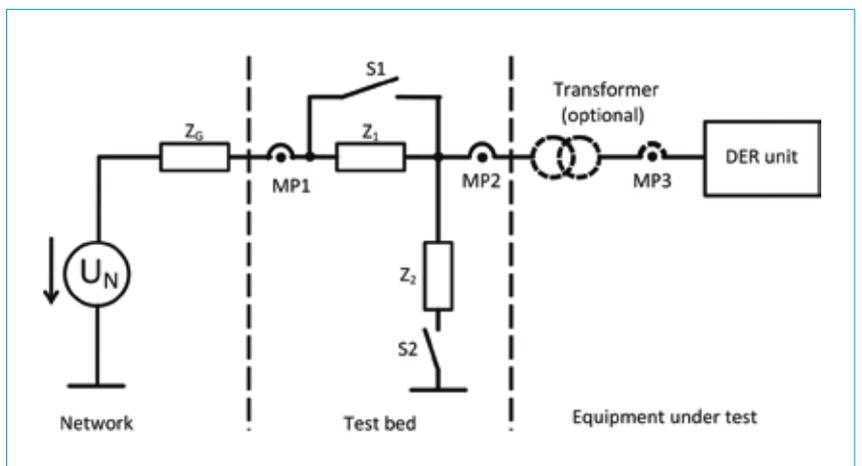
Figure 5. Simplified schematic of the LVRT container according to FGW TR3.
