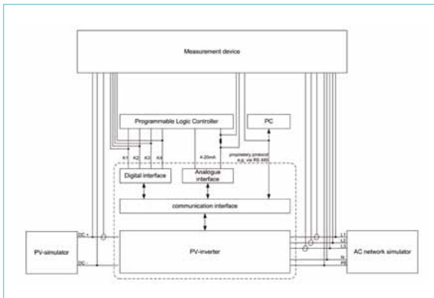
Figure 2. General measurement set-up of a PV inverter for measurements according to FGW TR3.
