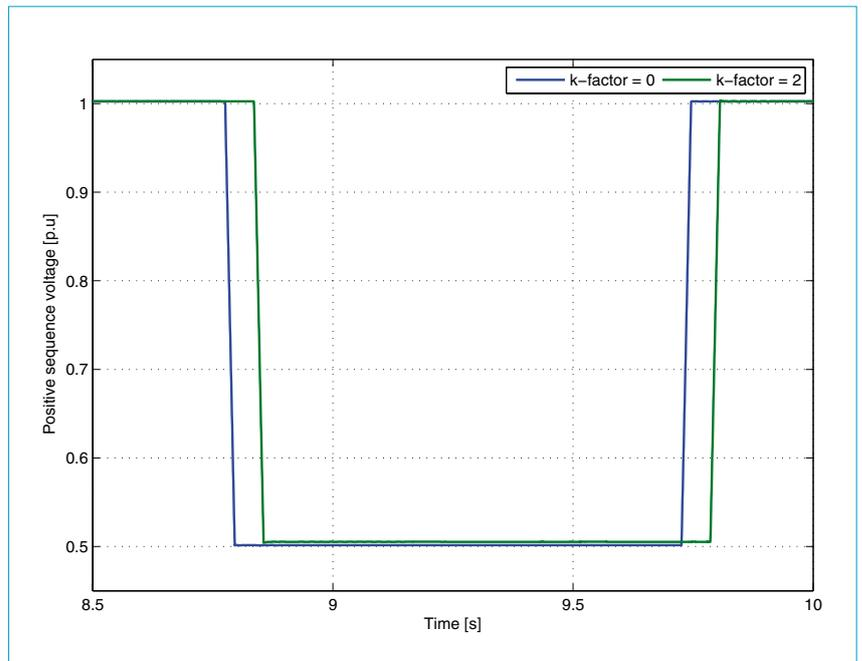
Figure 12. Influence of reactive current injection during network faults. The same voltage dip is applied to the PV-inverter (STP15000TL) in both cases.
