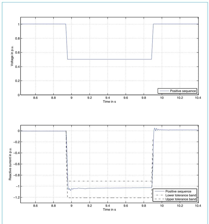
Figure 13. Measurement results for the STP 15000TL, when a balanced voltage dip to 50% of the nominal voltage  $U_n$  is applied.
