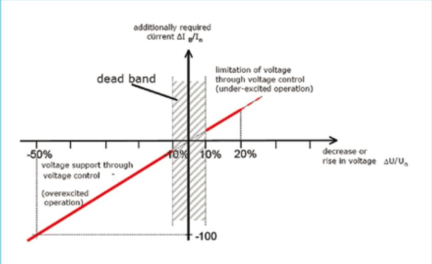
Figure 11. Reactive current injection from DER units during balanced network faults, according to [7].
