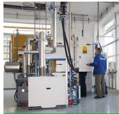
PE-CVD reactor for thin layers.
