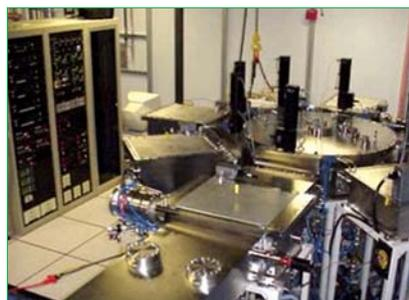
MVSystems' cluster tool for prototype production (PECVD and sputtering).
