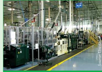
Uni-Solar's massive PECVD tool deposits the key thin-film ingredients in its amorphous-silicon process.
