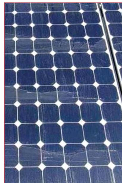
**Figure 6. Fielded modules with silicon contamination on glass surface show four stripes.**
