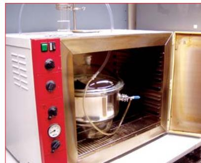
**Figure 1. Setup for highly accelerated ammonia life test. The desiccator was filled with an ammonia solution designed to produce an ammonia concentration of 50,000ppm at 85°C, as well as various materials used in PV modules, such as glass/EVA laminates, cables etc. that do not come into contact with the liquid ammonia solution.**
