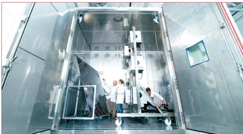
Figure 5. Large climate chambers conform to IEC standards at Fraunhofer CSP.
