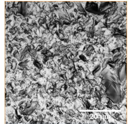
Figure 3. Surface of slurry wire sawn silicon wafer.
