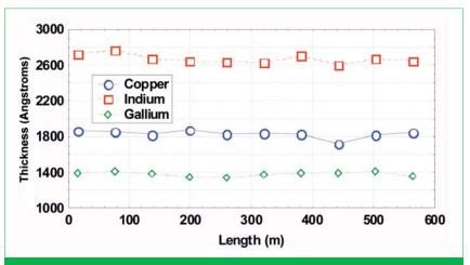
Figure 6. Equivalent thicknesses of copper, indium, and gallium in a CIGS film (down the web length) as measured by ex-situ XRF at the web centre.
