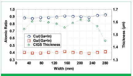
Figure 5. Atomic ratios and thickness of a CIGS film (across the web width) as measured by ex-situ XRF.
