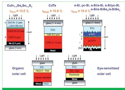
Figure 2. Typical variety of materials and cell structures used in thin-film technology. Many steps - such as TCO – require sputtering for correct deposition.
