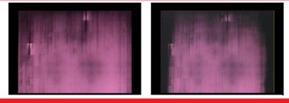
Figure 4. EL photography applied to a-Si modules, showing initial state (left) and after 1000h of damp-heat treatment (right – considerable reduction of photovoltaic active areas due to TCO corrosion (see TCO corrosion section overleaf).
