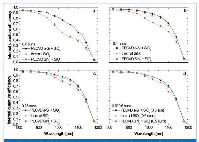
Figure 5. Comparison of bias light-dependent IQE measurements in the long wavelength regime of solar cells with (i) a-Si:H +  $a-SiO_x$ :H passivation, (ii) thermally-grown SiO<sub>2</sub> passivation, and (iii)  $a-SiN_x$ :H +  $a-SiO_x$ :H passivation on the rear [16].
