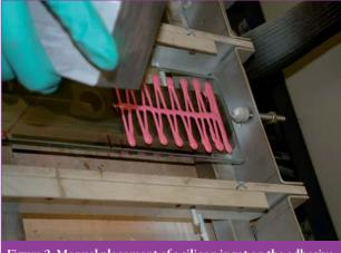
Figure 3. Manual placement of a silicon ingot on the adhesive.
