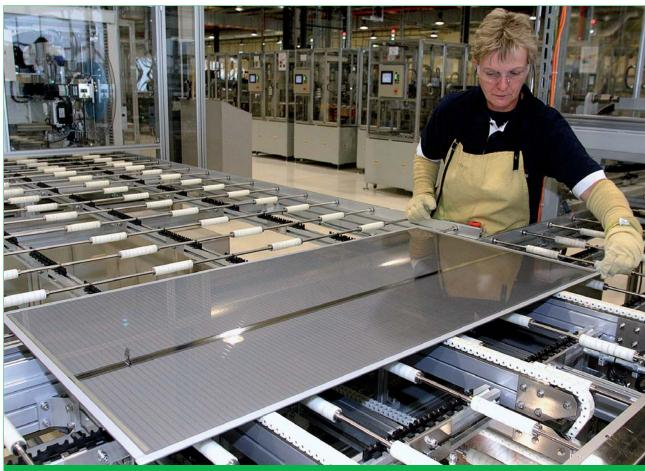
A CdTe module comes off the assembly line at First Solar's Perrysburg, OH, production plant.
