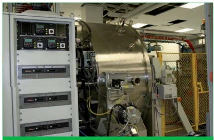
Figure 8. Front-electrode deposition by sputtering (a similar tool is applied for the back electrode).
