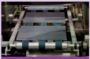
Figure 5. Wafer after separation (Fraunhofer IPA)
