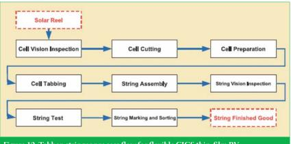
Figure 12. Tabber-stringer process flow for flexible CIGS thin-film PV.
