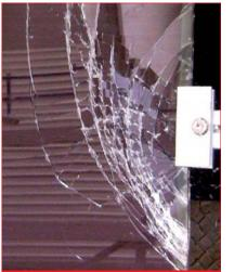
Figure 1. Breakage at 2,400 Pa: a-Si 1.4m<sup>2</sup> module with 2mm x 3mm glass.
