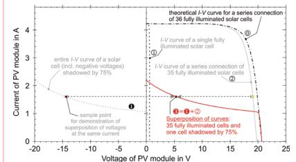
Figure 3. I-V curves showing a fully illuminated module (O); an illuminated module with one cell less (O); a shadowed cell (O); and the resulting I-V curve of a module with one shadowed cell (O).
