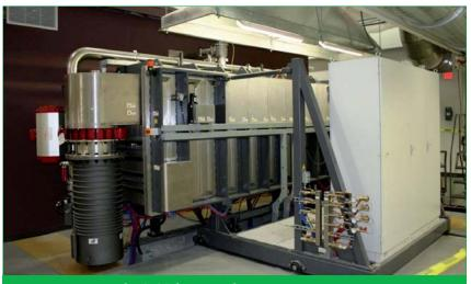
Figure 3. Equipment for CIGS deposition by coevaporation.
