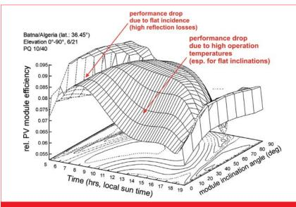
Figure 11. Results of simulation of a PV module. Image shows course of PV conversion efficiency during a day as a function of inclination angle of the module.
