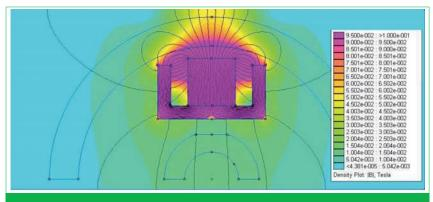
Figure 5. Electromagnetic simulation of rotary magnetron without optimization.
