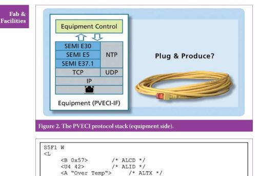
Figure 3. SECS-II example message (alarm: consists of alarm severity, alarm ID and alarm text).
