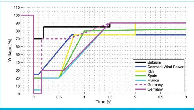
Figure 2. Requirements in national grid codes for decentralised generators connected to the distribution system during a grid fault.
