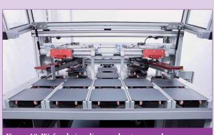
Figure 10. Wafers being dispersed onto several conveyors (AMB).
