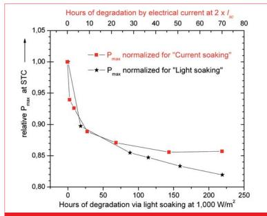
Figure 12. Comparison of degradation of an a-Si PV module via light soaking and via current (twice  $I_{SC}$ ).
