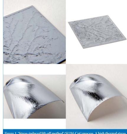
Figure 1. 'Stress-induced lift-off method' (SLIM-Cut) process. A high thermal stress is induced by a metallization layer, resulting in the release of a 50 $\mu$ m Si foil. The top row shows the remaining substrate and the bottom row, the thin lifted-off silicon layer.
