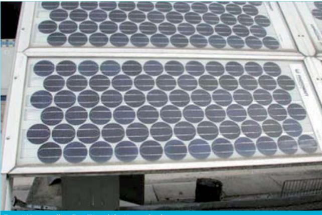
Figure 9. Monocrystalline silicon PV panel after 20 years of outdoor exposure.
