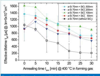
Figure 2. Carrier lifetimes of symmetric  $(SiO_x)$  a-Si/c-Si/a-Si  $(/SiO_x)$  samples after stepwise annealing. a-Si + SiO<sub>x</sub> systems show best stability [16].
