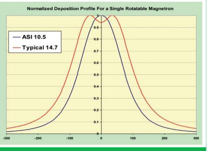
Figure 7. Rotary magnetron with optimized fields (blue line) directs more target material at substrate than un-optimized rotary magnetron (red line).
