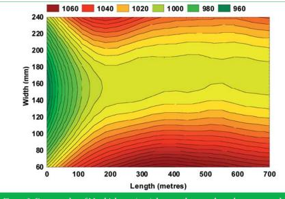
Figure 2. Contour plot of Mo thickness (a.u.) down and across the web as measured by XRF (distance weighted least squares fit).
