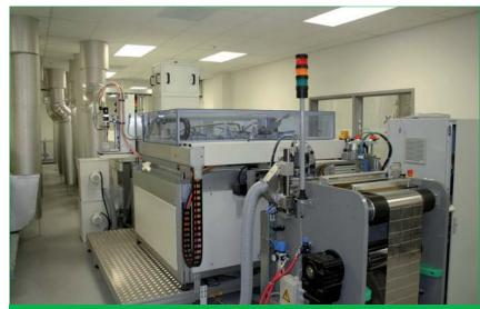
Figure 9. Collection grid printing system for CIGS cells.
