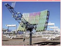
Atlas offers ultra-accelerated exposure testing system without overheating
