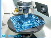
Laser ellipsometer and spectroscopic ellipsometer for measurement of thickness and refractive index of AR coatings on textured multi-crystalline and monocrystalline silicon wafers
