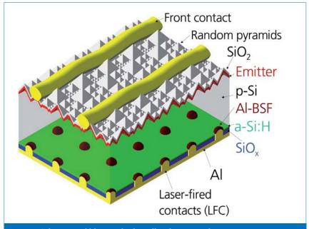
Figure 3. Schematic of fabricated solar cells. The rear surface passivation was created using a stack of PECVD a-Si:H and PECVD a-SiO,:H.
