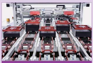
Figure 11. Wafer in stacker buffer (AMB)
