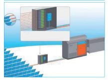
Satcon's 'Solstice' distributed energy management system designed for largescale PV power plants
