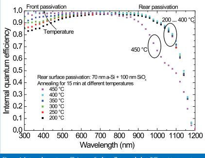
Figure 4. Internal quantum efficiency of solar cells annealed at different temperatures vs. the wavelength of light. An increase in front passivation (thermally-grown SiO<sub>2</sub>) at short wavelengths with annealing temperature was found. The rear passivation (a-Si + SiO<sub>x</sub>) is stable until 400°C but decreases strongly at 450°C [8].
