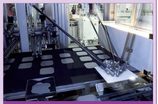
Figure 6. Wafer being transferred and sorted (Solarworld/ OregonDOT).
