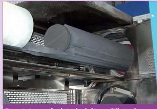
Figure 8. A quartz bot being loaded into a diffusion furnace (SEMCO).
