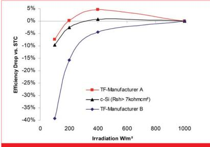
Figure 6. Change in power output as a function irradiance level for PV modules based on crystalline and thin-film technologies.
