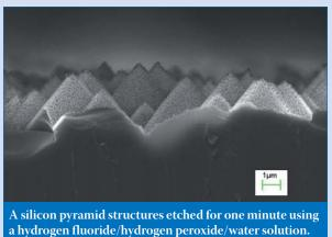
a hydrogen fluoride/hydrogen peroxide/water solution. The resulting structure has roughness at the micron and nanometre scales.
