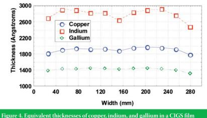
(across the web width) as measured by ex-situ XRF.
