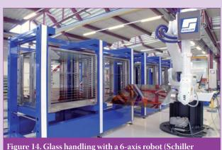
Figure 14. Glass handling with a 6-axis robot (Schiller Automation).
