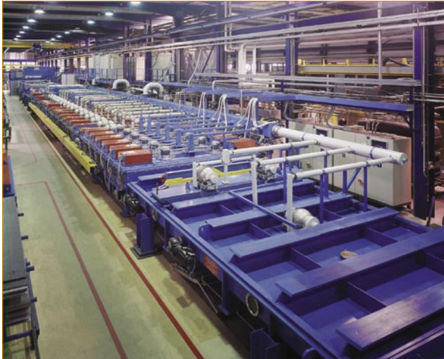
Figure 4. Sheet glass used for solar cells is manufactured on several float glass units, each of which is one hundred metres long.
