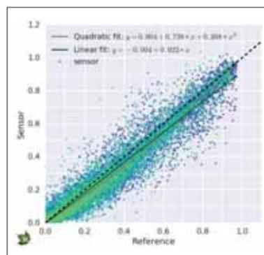
**Figure 3. Sensor irradiance versus satellite-based reference irradiance with linear and quadratic regression; the slope is 8% too low; 860 kW site in Belgium, data from 1 June 2015 (blue) to 31 May 2016 (green), orientation 30° south**
