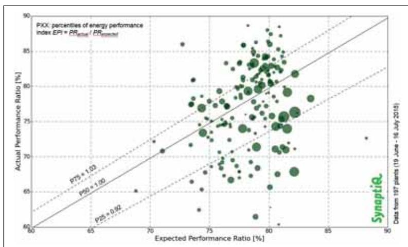
**Figure 1: Actual performance ratio (PR) from monitoring versus expected PR based on plant specification and real weather data for 197 PV plants in Europe; the worst 25% perform more than 8% below expectation; the dot size represents the size of the PV plant**
