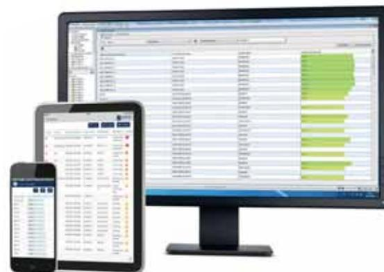
plant. The graphical display can be sorted according to the performance ratio of each individual device. In this way, any poorly performing inverters become immediately obvious. Added to this, the alarms from all power plants under supervision can be brought together and processed in a single place.
