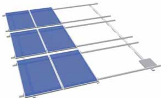
of mechanical attachments or counterweights over the roof ridge. A special ridge angle joint has been designed for installations on pitched roofs, which can be easily adapted to each site specific situation. The system solution was designed to meet the specifications of snow loads up to 50psf and wind speeds up to 130mph. Ballast stone clamps are available for installations
