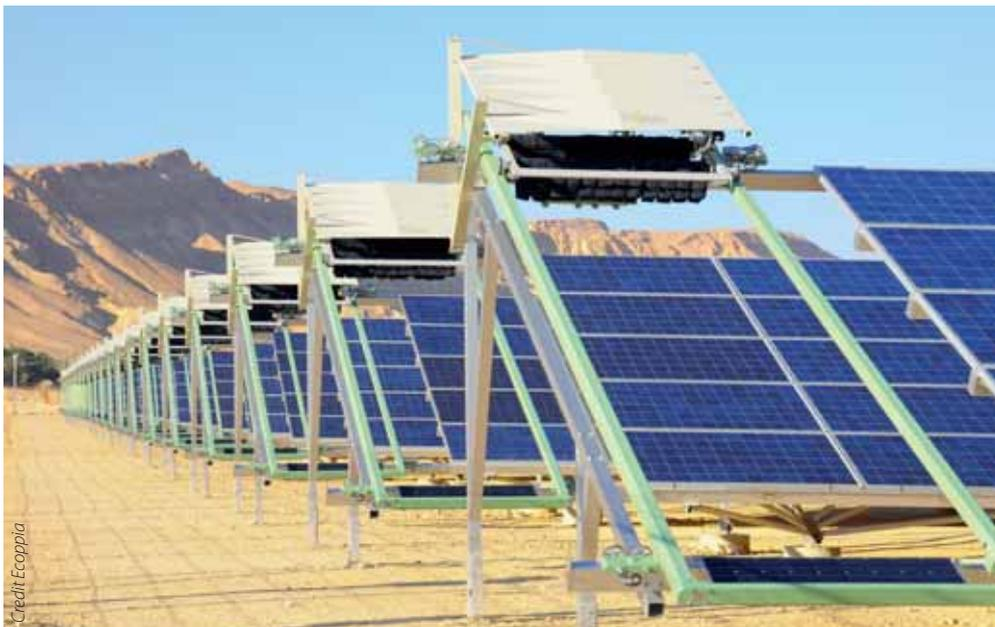
ing a specially designed soft brush that minimises the abrasion visited on the module. Another advantage of automated cleaning he says is its responsiveness to sudden soiling events such as sand or dust storms. Ecoppia's solution is operated via the cloud, with sensors at the site keeping a constant check on particulate levels, and issuing instructions to clean if they pass a certain threshold. That means cleaning can be underway in next to no time.
