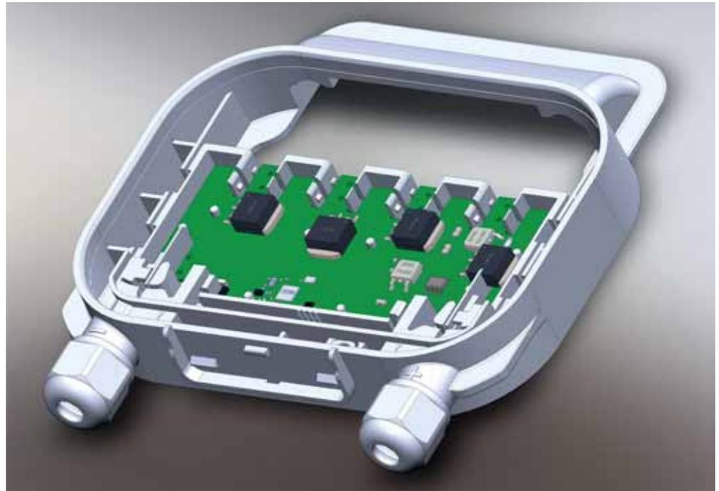
**Platform:** The SunSniffer sensor measures voltage and temperature at each single module, and the simulation engine in combination with artificial intelligence allows the system to detect even the smallest error – with an accuracy of under 1%, according to the company. The
