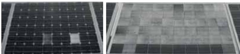
**Figure 3:** electroluminescence images from PID-affected modules in field: 'surface' PID (left) and 'frame' PID (right) depending on different leakage current distribution in PV modules [1]
